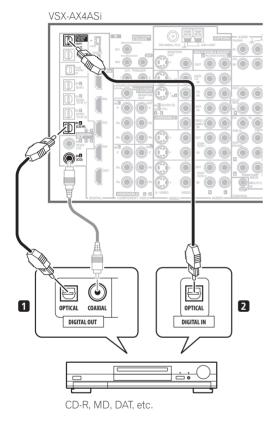
1 Connect an optical-type<sup>1</sup> digital audio output on your digital component to the DIGITAL 4 (CD-R) input. Use an optical cable for the connection.
